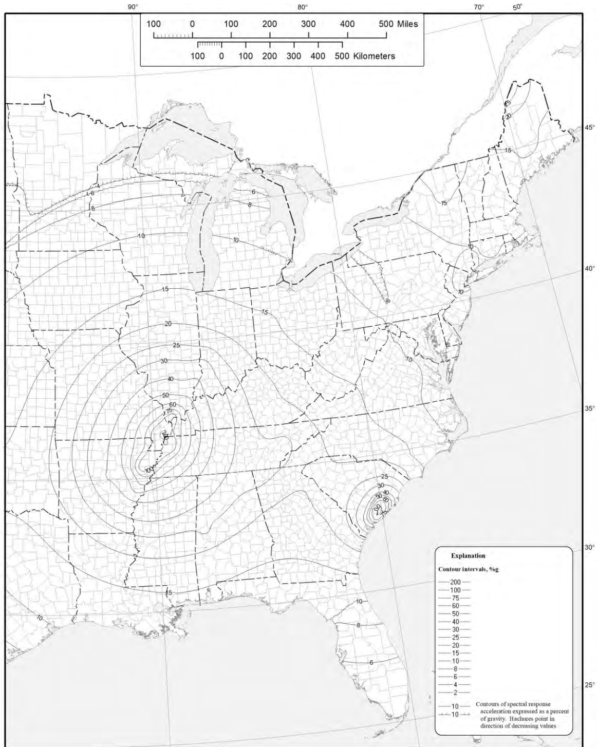
Figure 22-2 (continued) S_{M1} for the Default Site Class, for the Conterminous United States
