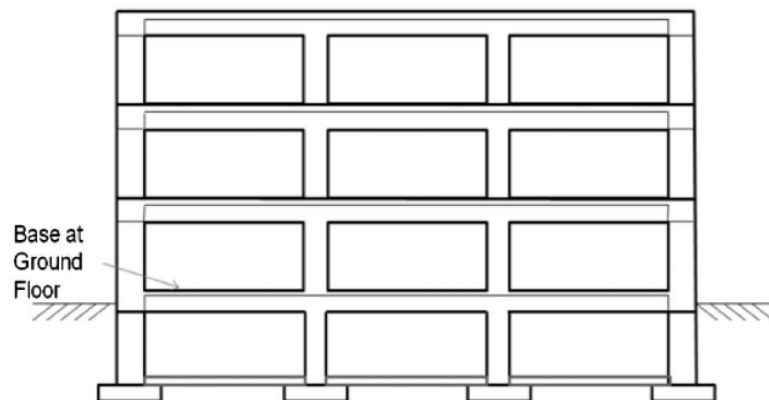
FIGURE C11.2-3 Base at Ground Floor Level
